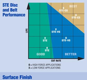
STE-CS – aggressive, closed structure, very sharp; works best on harder materials, low-and high-force applications.
