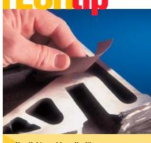
Use light machine oil with cloth rolls as a lubricant for finer finishes and quicker cut.
